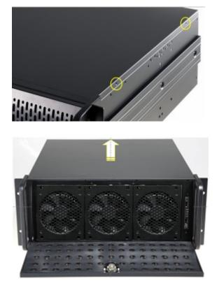
Remove the screws from each side of the Chassis. (two on each side)
